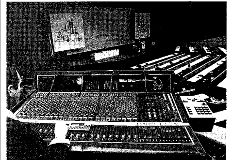
This Studer 900 mixing console is part of the infrastructure of the CCH (Congress Center Hamburg). This was incidentally one of the first Series 900 mixing console ever delivered.
